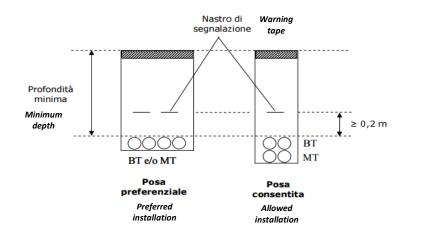
More pipes can be laid into the same trench, according to the layout in side figure
